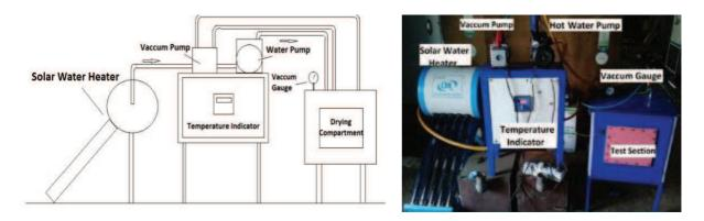
Figure 8. Various component of vacuum solar drying system (Thigale and Patil, 2016)
