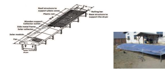
Figure 5. Schematic diagram and photo of solar tunnel dryer (Bala and Janjai, 2009).
