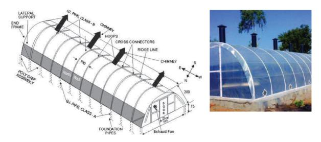
Figure 6. Walk-in type hemi-cylindrical solar tunnel dryer (Rathor and Panwar, 2010).
