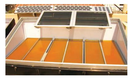
Figure 2. Highly efficient direct cabinet solar dryer (Rao, 2014).
